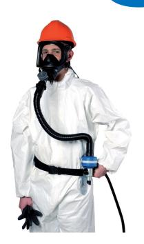
The **TR 82** full face mask with panoramic visor is connected to the overflow valve that releases the excess air to the external environment. The mask is fed by the **TUR 60** corrugated hose which droves breathable air in the respiration zone and which is positioned between the overflow valve and the filter silencer connected to the flow regulator.
